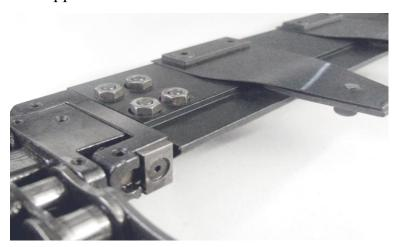
The grippers are made of special extra hard aluminum alloy, with anode treatment on the surface, ensuring accurate die cutting and embossing, ect. at high speed. The adjustment mechanism, patent design guarantees very accurate control. An imported chain is used for the main gripper transmission, with strength increased by 45% for accurate stability and prolonged life.
