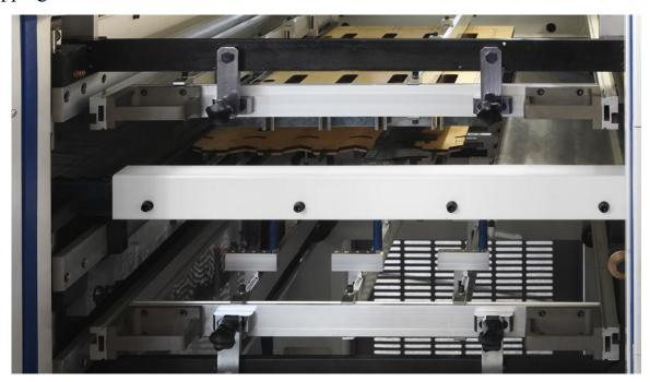
A triple-interlocked-piece stripping device, action harmony, precision effectively, can effectively remove all kinds of special waste
