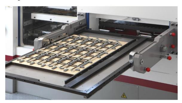
The driving gear ensures high speed of die cutting together. The pneumatic locking mechanism and air clutch are fast and stable. The die cutting frame can prevent the die cutting plate from drooping or separating effectively.
