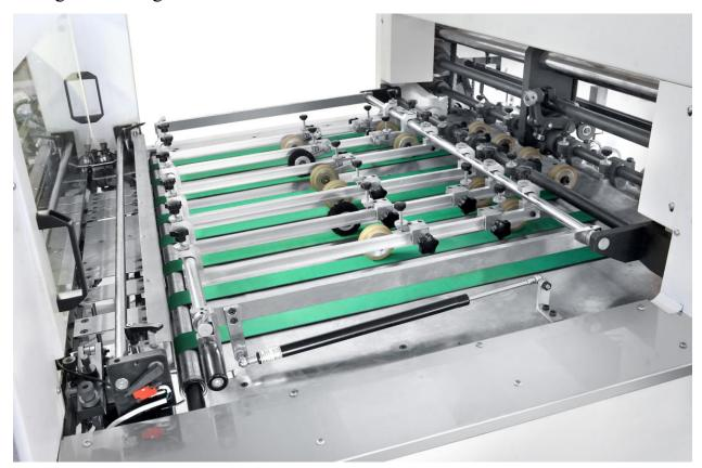
The incline-type paper moving table top is more suitable to high-speed thin paper and location. Side location adopt dual purpose side device with pull guide and push guide, accounting to paper choose, it makes switch easier. It could switch front rise position arriving reduction of speed device, it is benefit of thin paper's location.
