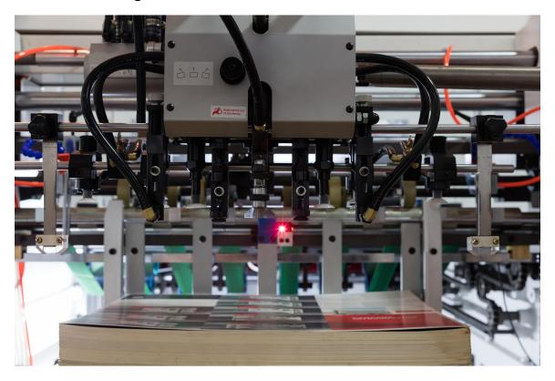
The design of stacker preparatory stage was improved, it could use prepared car sheet piling. Also could use ordinary hydraulic car sheet piling to stacker directly. The machine has four suction nozzles and four sending nozzles in feeder, ensure feed smoothly. Adopt import screw air-blowing device, it could make the sheet send smoothly.
