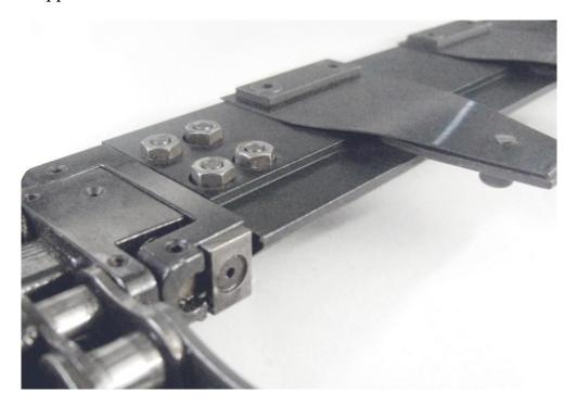
The grippers are made of special extra hard aluminum alloy, with anode treatment on the surface, ensuring accurate die cutting and embossing, ect. at high speed. The adjustment mechanism, patent design guarantees very accurate control. An imported chain is used for the main gripper transmission, with strength increased by 45% for accurate stability and prolonged life.
